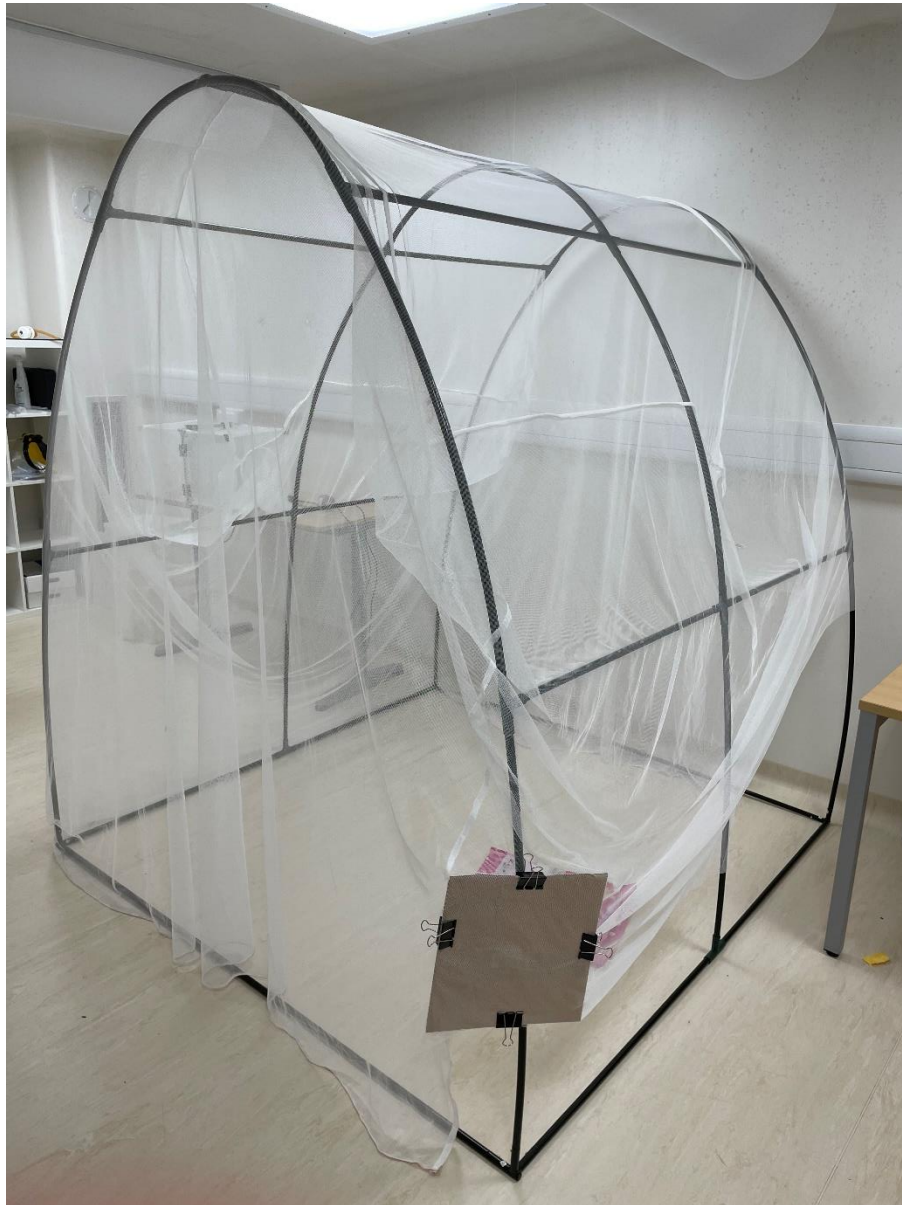
Figure 1 - Frame (a Walk in Tunnel Greenhouse, 181 x 181 x 200cm) for hanging a full net for airing and breakdown of panels.
